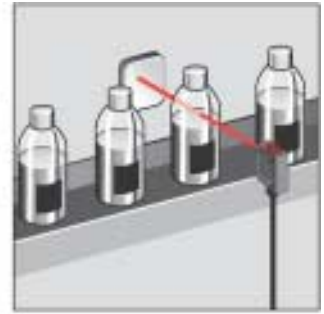
BOS 6K-... Retroreflective with low hysteresis
